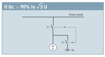
Io: motor off-load current U: supply voltage
