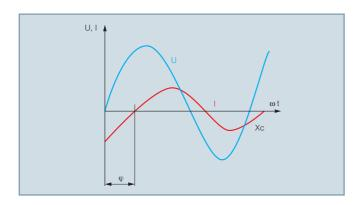
This energy, which is generally expressed in kilovolt-ampere-hours (kVAh), corresponds to the apparent power S (kVA) and can be broken down as follows:
