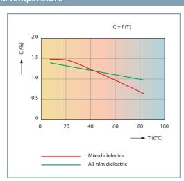
In comparison with the previous generation of "mixed" type dielectric (paper + film) capacitors, synthetic "all-film" type dielectric capacitors have a much longer service life, due to:
