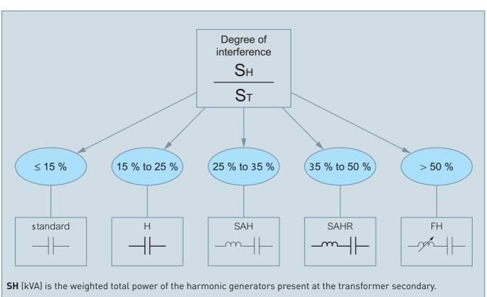
**ST** (kVA) is the power rating of the HV/LV transformer.
