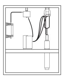
• Possible components: damping reactors, discharge reactors, contactors, HRC fuses, power factor relays, detuned reactor, etc.
