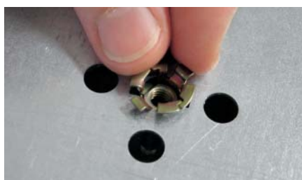
Remove the plastic cover at the rear of the enclosure and fit the clip-nut
